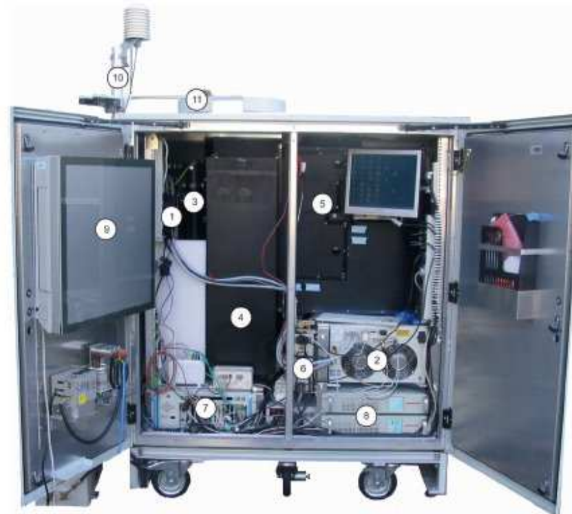
FIG. 2. Cabinet with open doors showing the major parts of the Raman lidar system Polly XT : (1) laser head, (2) laser power supply, (3) beam expander, (4) receiver telescope, (5) receiver with seven channels, (6) power supply for PMT cooling unit for the 1064-nm channel, (7) computer with data acquisition and interface cards, (8) UPS, (9) air conditioner, (10) sensors for outdoor temperature and rain, and (11) roof cover.
