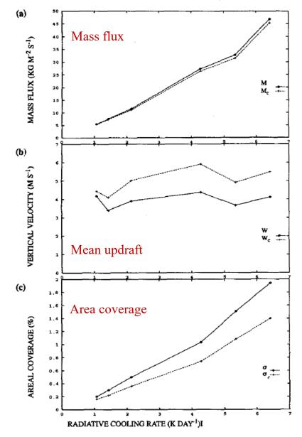
Fig. 7. Time mean of cloud properties at 6.75 km of altitude, plotted as a function of the cooling rate, R, and logarithmic curve fits. (a) Upward cloud mass flux M and convective mass flux  $M_c$ . (b) Mean upward velocity  $\overline{w}$  and mean convective velocity  $\overline{w}_c$  in the clouds. (c) Areal coverage of cloudy updrafts  $\sigma$  and of convective updrafts  $\sigma_c$  (units are in percentages of the total area).
