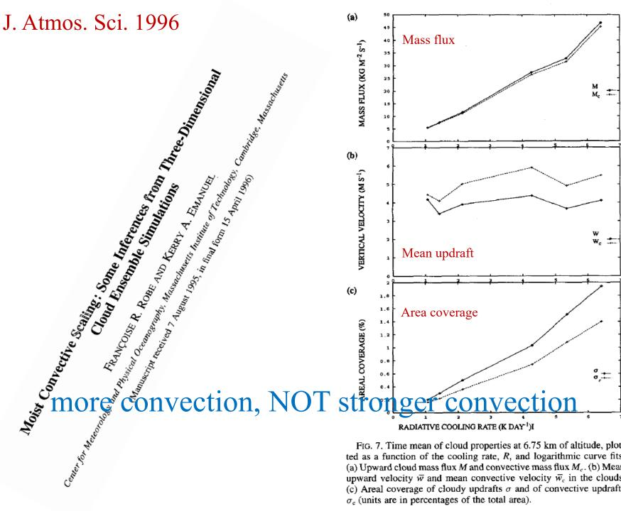
Fig. 7. Time mean of cloud properties at 6.75 km of altitude, plotted as a function of the cooling rate, R, and logarithmic curve fits. (a) Upward cloud mass flux M and convective mass flux  $M_c$ . (b) Mean upward velocity  $\overline{w}$  and mean convective velocity  $\overline{w}_c$  in the clouds. (c) Areal coverage of cloudy updrafts  $\sigma$  and of convective updrafts  $\sigma_c$  (units are in percentages of the total area).
