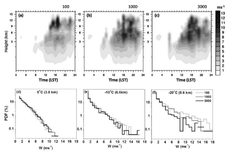
FIG. 11. (top) Time evolution of vertical profiles of simulated maximum updraft in the selected study region for CCN concentrations of (a) 100, (b) 1000, and (c) 3000 cm<sup>-3</sup> where updrafts are greater than 1 m s<sup>-1</sup>. (bottom) PDFs (%) over the whole domain at (d)  $5^{\circ}$ , (e)  $-10^{\circ}$ , and (f)  $-20^{\circ}$ C during 1500–1800 LST are also shown.
