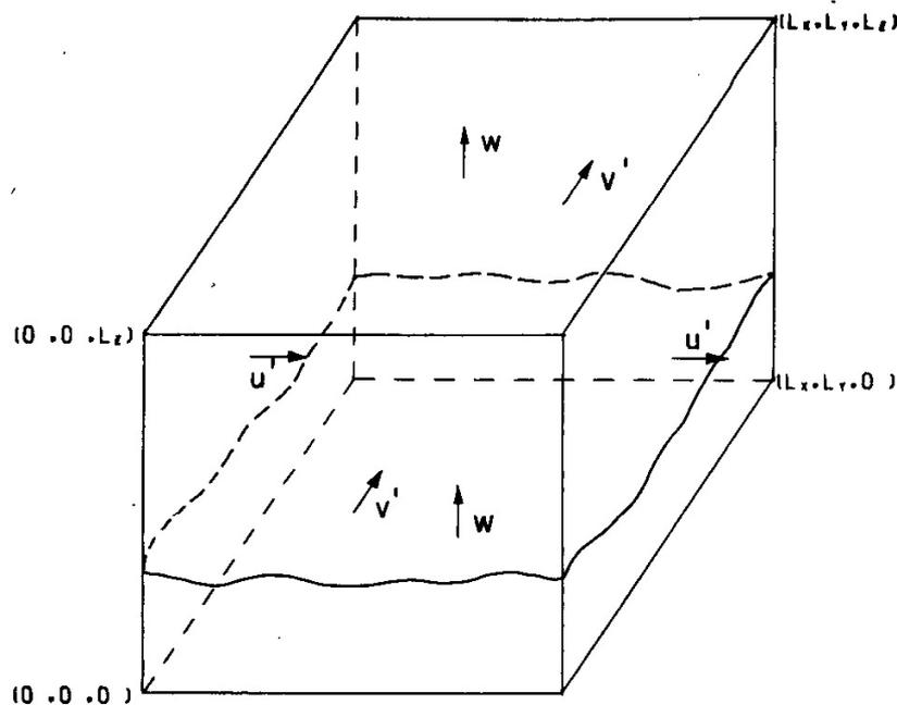
FIG. 1. Domain of integration.  $L_x = L_y = L_z = 200$  m. Subcloud region typically extends from  $z = 0-50$  m. Dry subcloud air is forced through the domain with a mean vertical velocity  $\bar{w}$ . Perturbation velocities  $u'$ ,  $v'$  and  $w'$  with zero horizontal averages are dynamically imposed on the flow.
