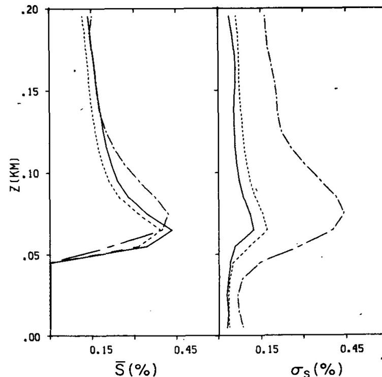
FIG. 3. Supersaturation profiles in units of percent for Runs 1, 2 and 3. Solid line: Run 1,  $CCl = 2000 \text{ cm}^{-3}$ ,  $\bar{w} = 2.0 \text{ m s}^{-1}$ ; short dashes: Run 2,  $CCl = 600 \text{ cm}^{-3}$ ,  $\bar{w} = 1.0 \text{ m s}^{-1}$ ; long and short dashes: Run 3,  $CCl = 100 \text{ cm}^{-3}$ ,  $\bar{w} = 0.5 \text{ m s}^{-1}$ .
