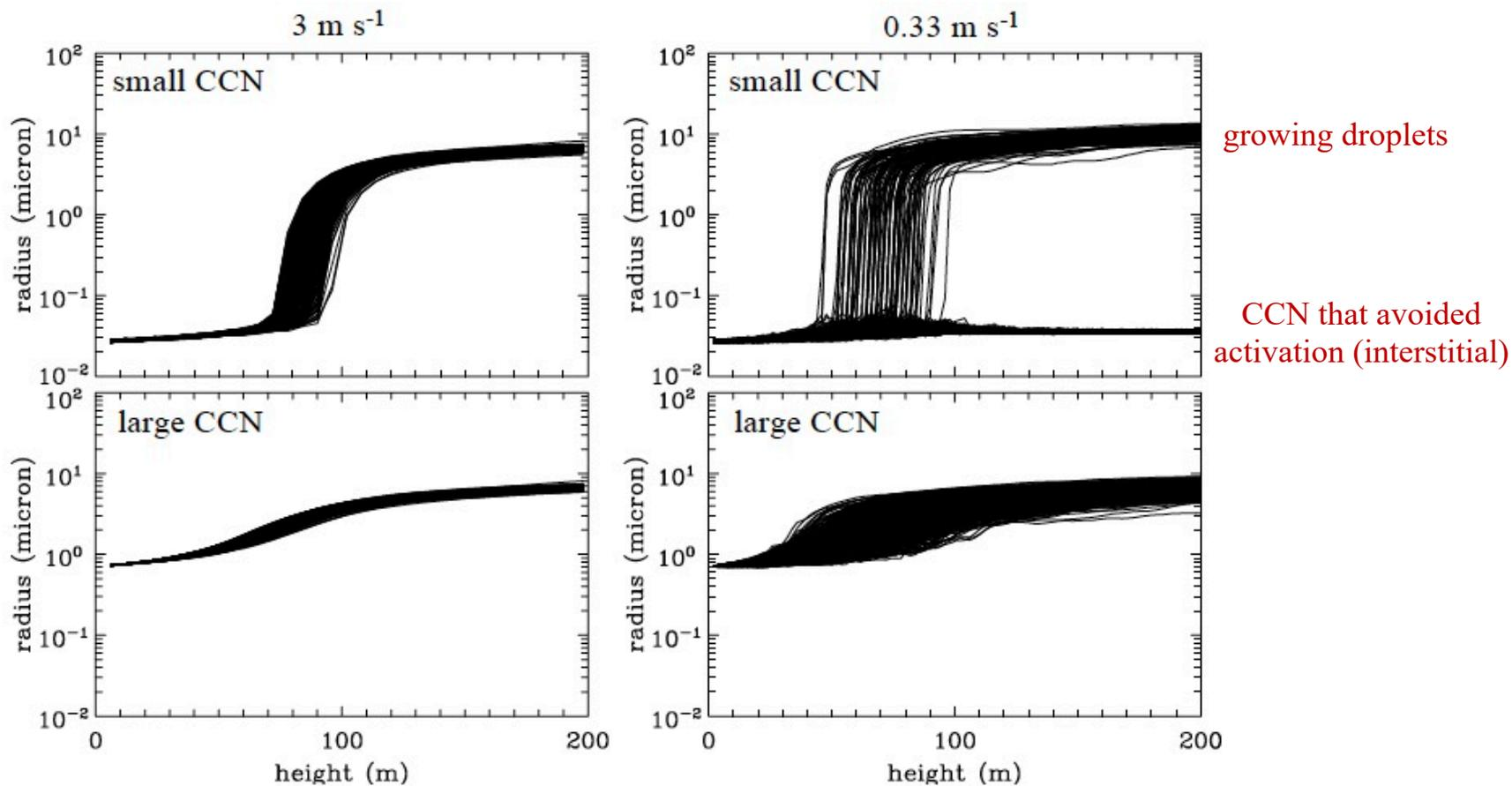
Finite spectral width comes from CCN activated at various times...
