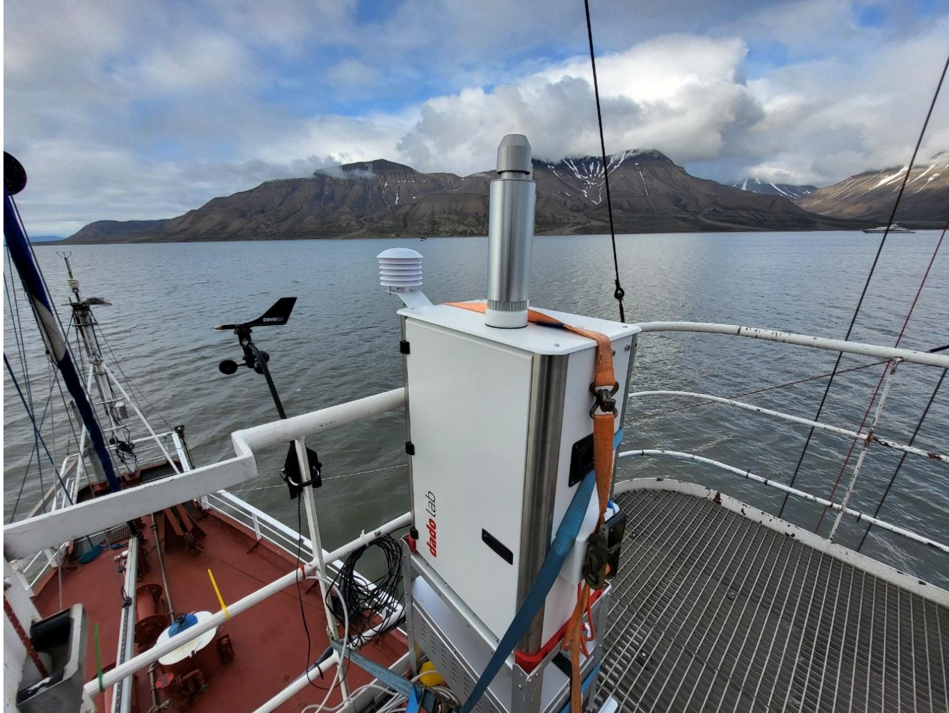
Aerosol aspirator DadoLab Gemini on board rv Oceania in Svalbard (Longyearbyen, Norway)
