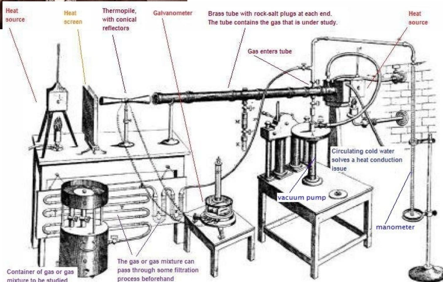
1861, Tyndall's apparatus measuring properties of greenhouse gases.
