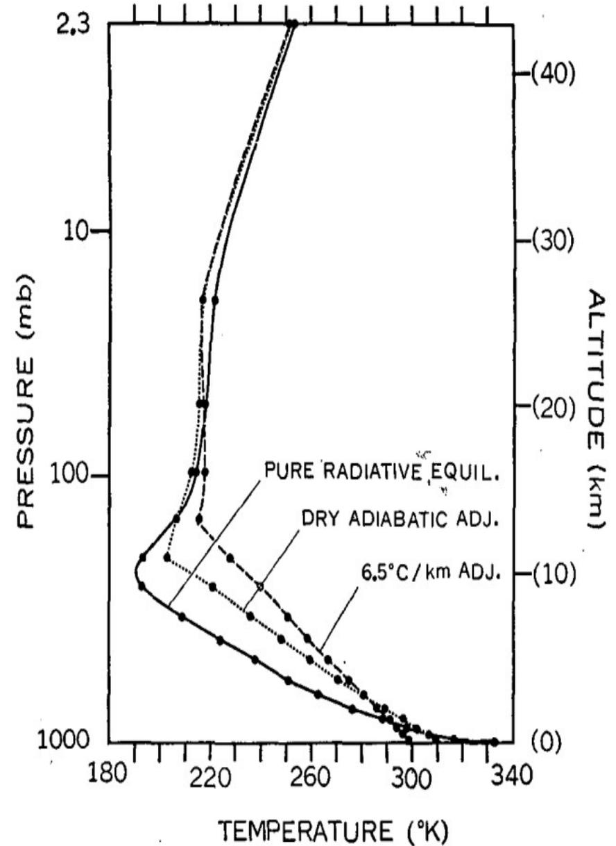
FIG. 4. The dashed, dotted, and solid lines show the thermal equilibrium with a critical lapse rate of  $6.5 \text{ deg km}^{-1}$ , a dry-adiabatic critical lapse rate ( $10 \text{ deg km}^{-1}$ ), and pure radiative equilibrium.
