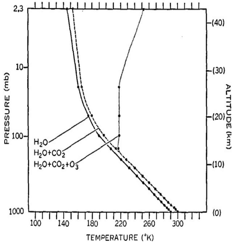
FIG. 6c. Thermal equilibrium of various atmospheres which have a critical lapse rate of  $6.5 \text{ deg km}^{-1}$ . Vertical distributions of gaseous absorbers at 35N, April, were used.  $S_c=2 \text{ ly min}^{-1}$ ,  $\cos \bar{f}=0.5$ ,  $r=0.5$ , no clouds.
