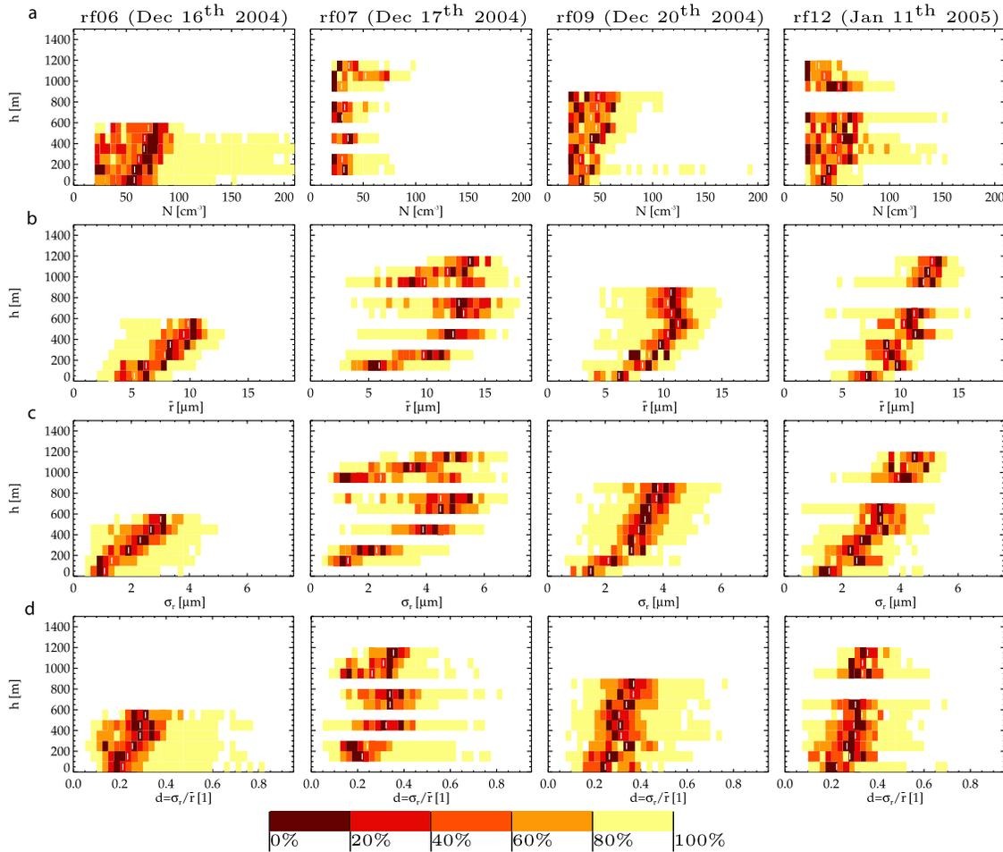
**Figure 1.** Statistics of droplet-spectrum and concentration measurements from RICO flights rf06, rf07, rf09, and rf12 as a function of height. (a) Droplet concentration  $N$ , (b) the mean radius  $\bar{r}$ , (c) the standard deviation of radius  $\sigma_r$ , and (d) the relative dispersion  $d = \sigma_r/\bar{r}$ . See text for details.
