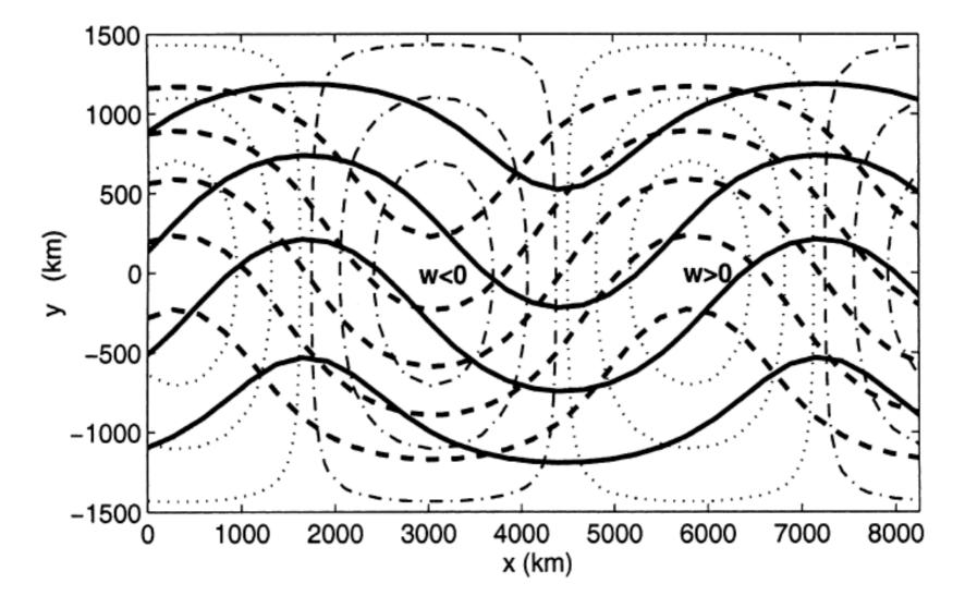
Schematic 500-hPa height contours (solid lines), isotherms (dashed lines), and vertical motion field (w > 0 dash-dot lines, w < 0 dotted lines) for a developing synoptic-scale system. Upward motion occurs where vorticity decreases moving left to right along an isotherm, and downward motion occurs where vorticity decreases moving left to right along an an isotherm.
