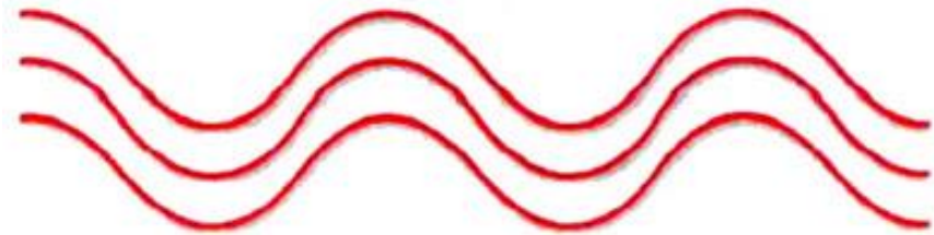
LASER: One color (monochromatic) and waves in phase (coherent)
