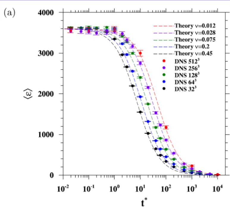
Energy dissipation rates as function of  $t^*$ . The model predictions are also shown with  $\beta = 0.8$ .
