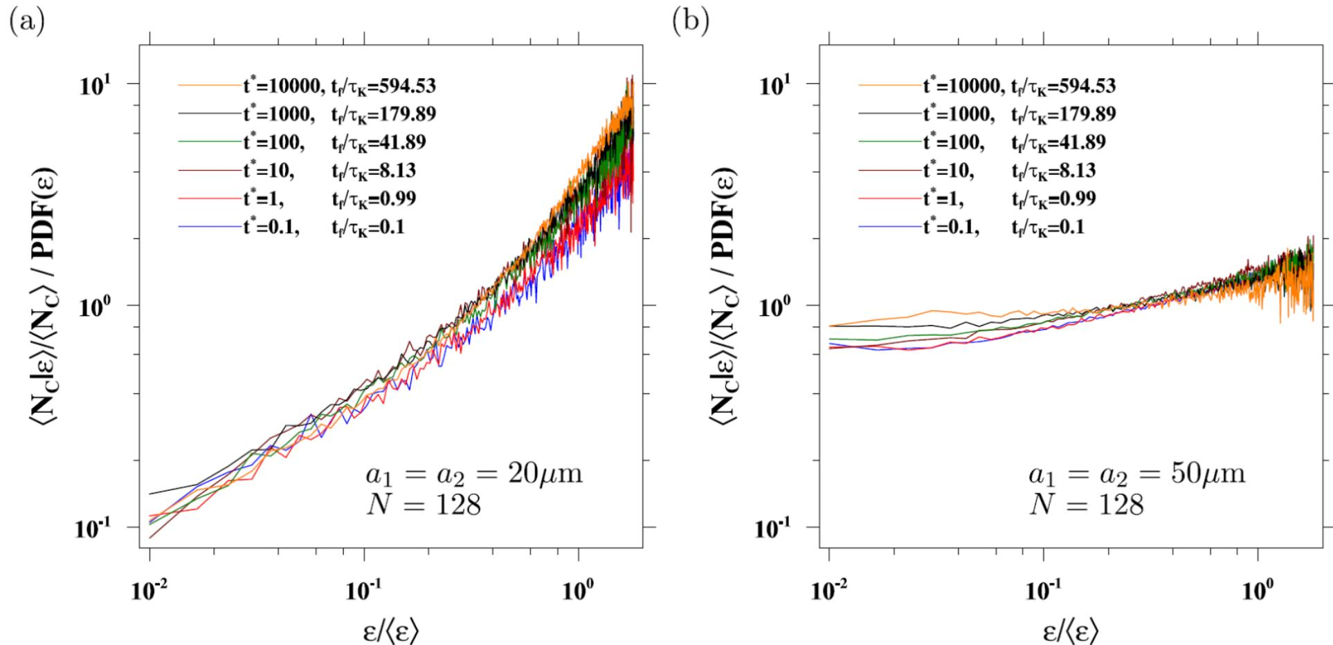
Correlation between the local collision rate and energy dissipation rate as a function of normalized energy dissipation rate. Panel (a) monodisperse systems with 20  $\mu\text{m}$  droplets; (b) monodisperse systems with 50  $\mu\text{m}$  droplets.
