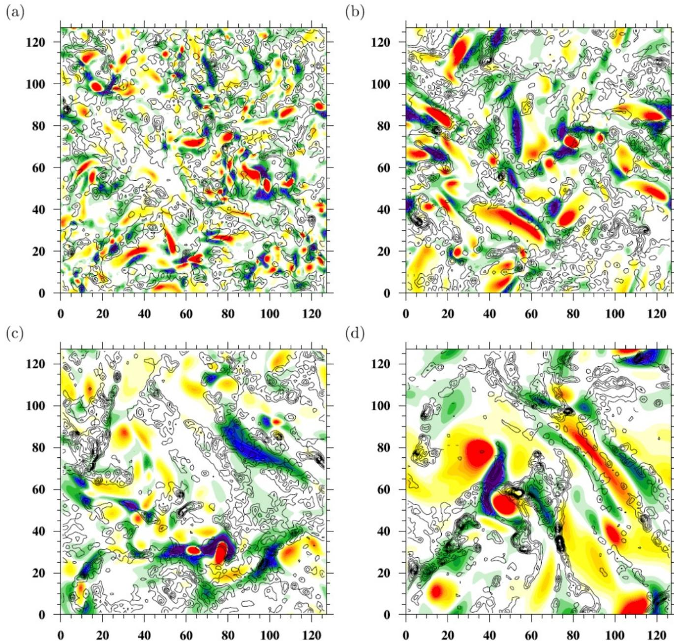
Black contour - distributions of particles with Stokes number of 0.254 (droplet radius  $a = 20 \mu\text{m}$ )
