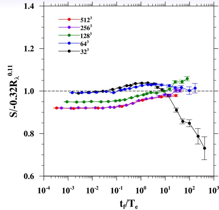
The integral length scale, flatness and skewness show a strong dependence on the forcing time scale when the scale is large, which could be a result of very low flow Reynolds numbers.
