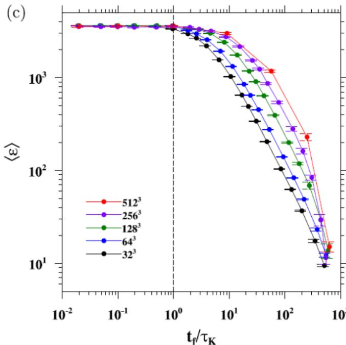
Panel (b) energy dissipation rate from DNS in log-log scale, with the x-axis being the forcing time scale normalized by eddy turnover time.
