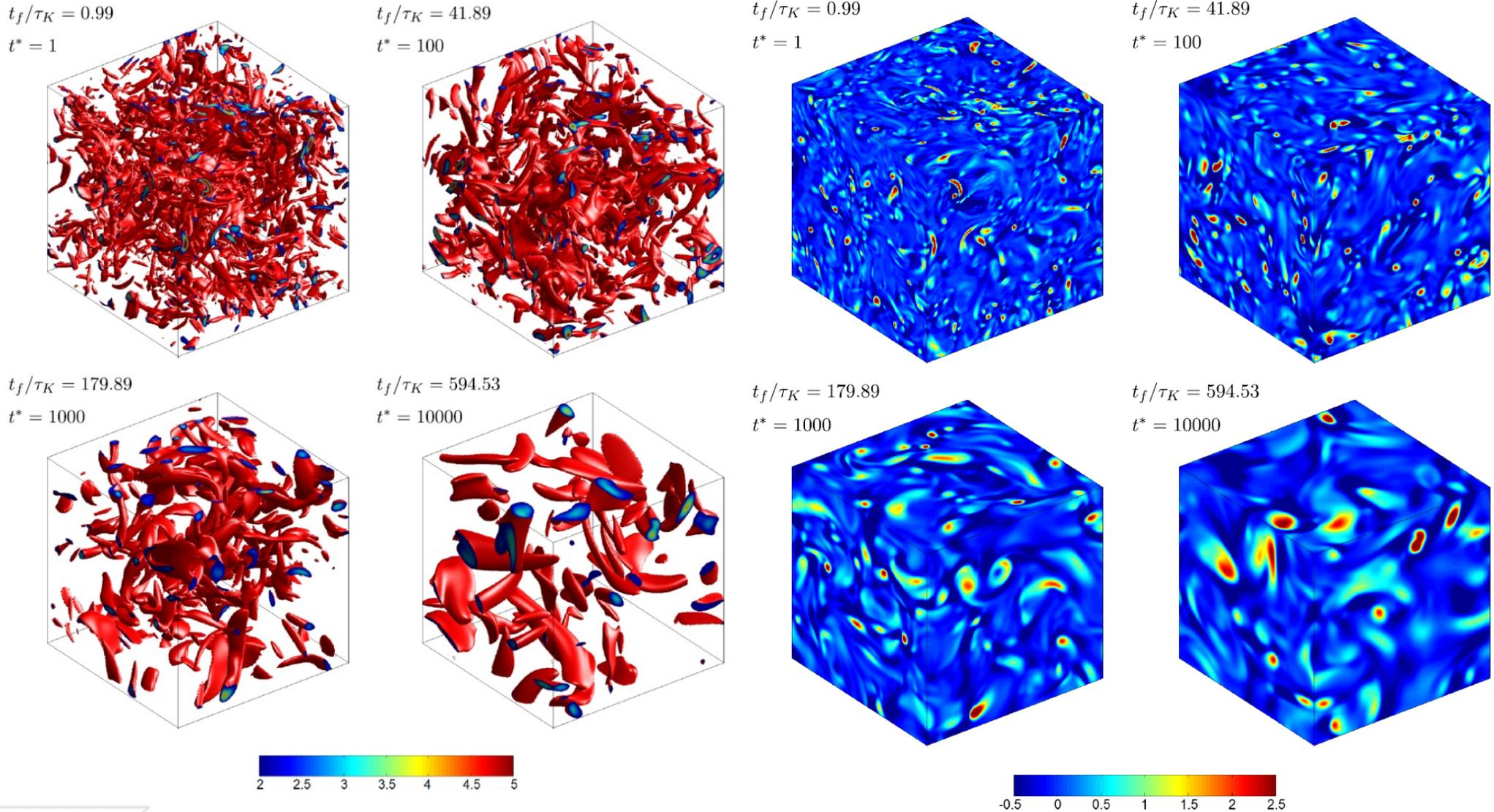
Vorticity isosurfaces (in red) and vorticity magnitude inside vortex structures at the boundaries of the domain (shown with color mapping) for the simulated flows with different forcing time scales ( $N = 128^3$ ).
