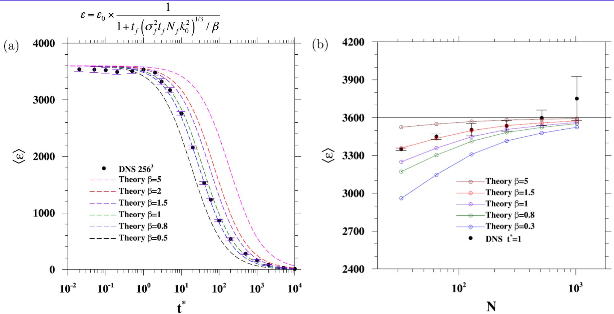
Panel (a) energy dissipation rates as a function of  $t^*$ . Markers represent results from DNS at resolution  $N = 256$ . Dashed lines - model predictions for different  $\beta$  values. Panel (b) energy dissipation rate from DNS (black markers) for  $t^* = 1$  at different resolutions. Color lines represent analytical predictions.
