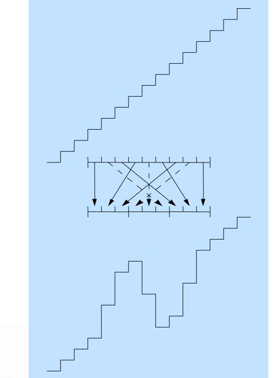
The triplet map is implemented numerically as a permutation of fluid cells.
