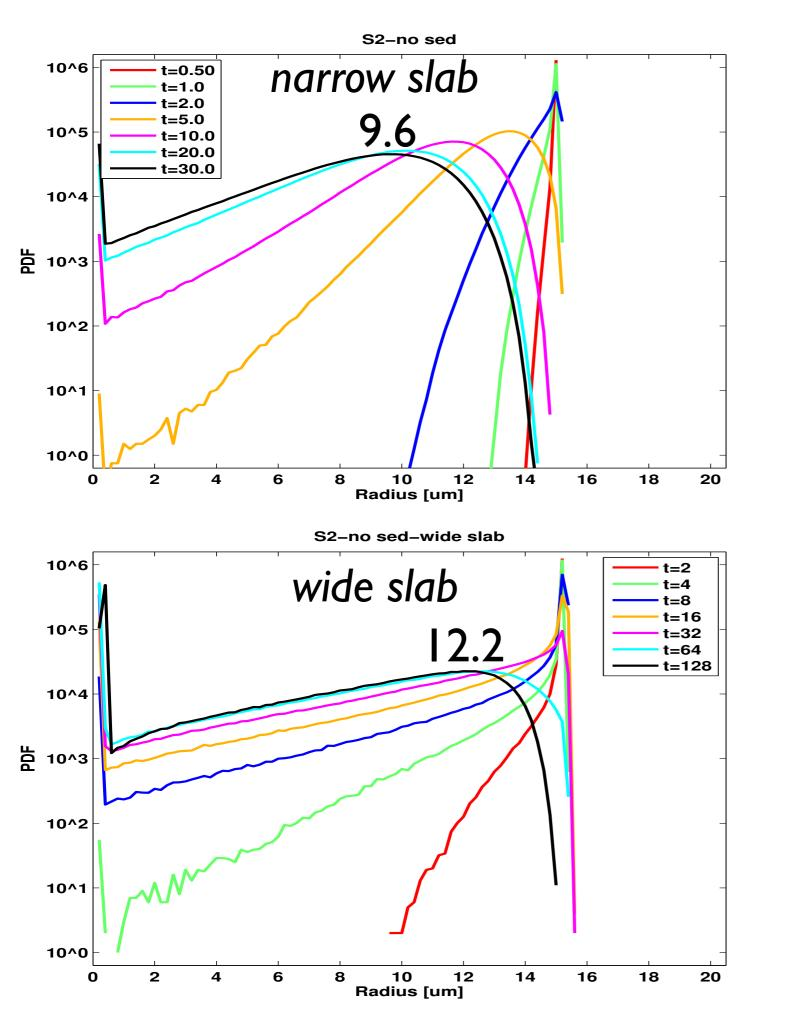
Initial droplet radius is 15 microns. Some droplets completely evaporate.
