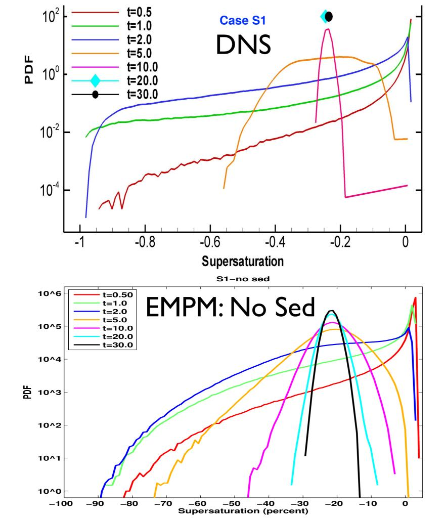
Super-saturation at droplets (including completely evaporated ones)
