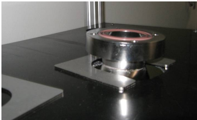
Figure 12 Installing the isokinetic flow splitter.
