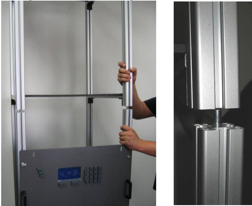
Figure 11 Attaching the top ACS rack section.
