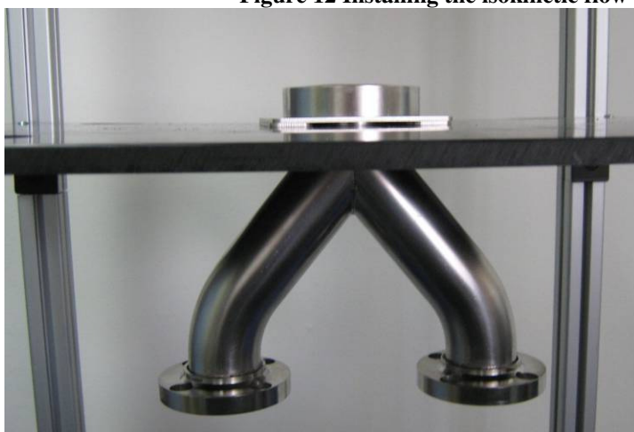
Figure 13 Secured isokinetic flow splitter.
