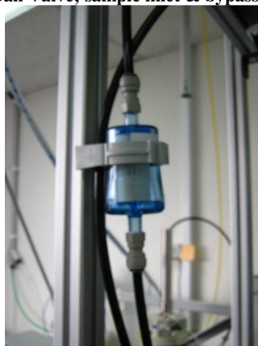
Figure 22 Bypass DFU in position
