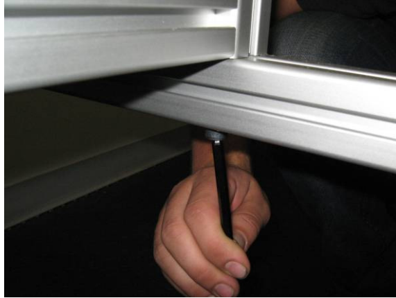
Figure 10 Securing the ACS rack to the instrument rack.
