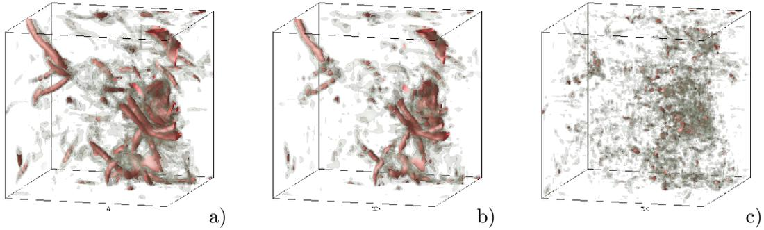
Figure 1: Homogeneous isotropic turbulence. Isosurfaces of vorticity modulus for a) total flow, b) coherent part, c) incoherent part.
