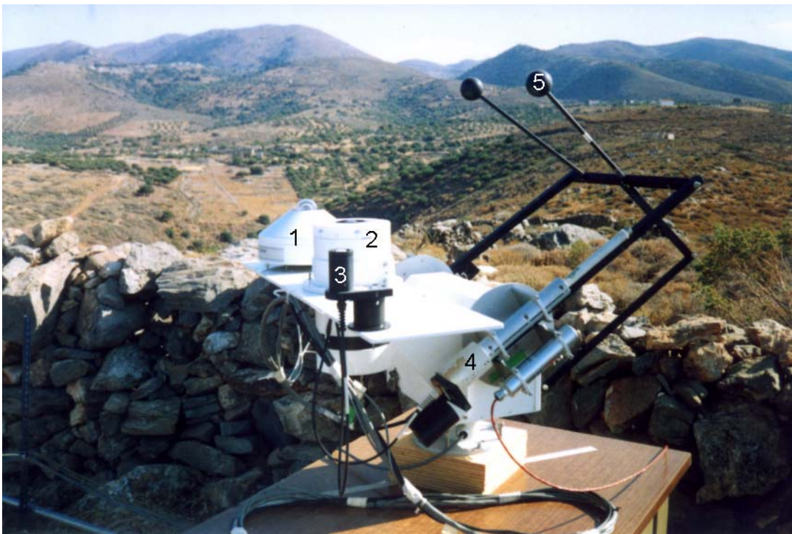
Fig. A1.2 Radiation instruments at the Finokalia station during MINOS experiment 2001. This picture shows sun tracker with (1) CM21 pyranometer, (2) GUV-511 Biospherical Instruments radiometers, (3) total flux analytical spectral device (ASD) diffuser, (4) tube with direct flux ASD diffuser, and (5) shading ball.
